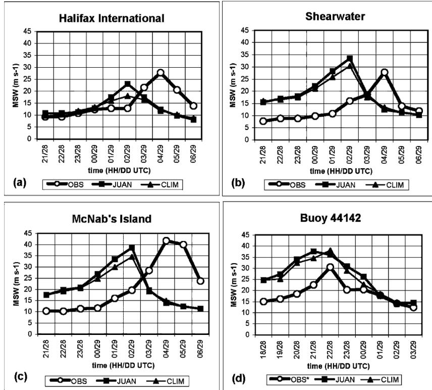
FIG. 10. Time series output of instantaneous surface wind speed from the model (valid at 40 m) and from weather stations (valid at 10 m) for various locations: (a) Halifax International Airport, (b) Shearwater, (c) McNab's Island (Halifax Harbour), and (d) buoy 44142 (~200 km south of storm landfall location).
