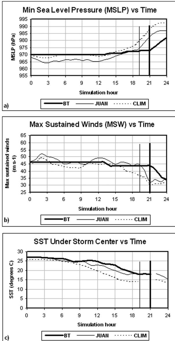
FIG. 7. Model results for the control simulations: (a) evolution of MSLP for JUAN (thin, solid), CLIM (dashed), and the BT (thick, solid); (b) MSW; and (c) SST beneath the storm center as a function of model simulation time (hours). Vertical lines indicate time of landfall for the simulations (thin) and BT (thick).
